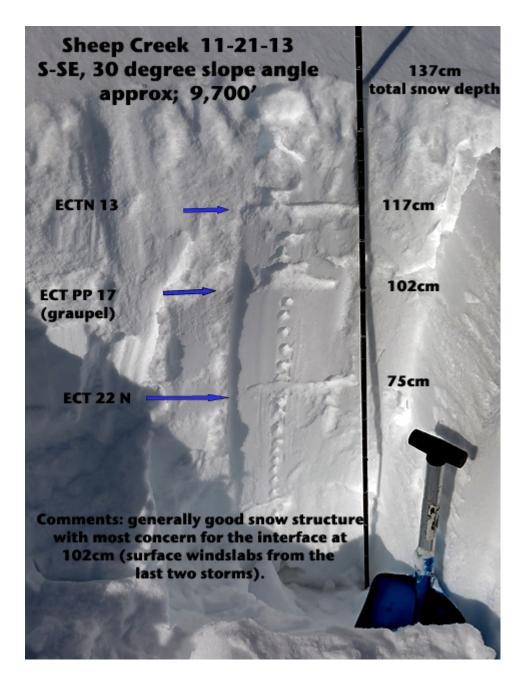
The snowpack is 4.5 feet deep in this photo and mostly stable. The weakest layer in the photo is labeled at 102 cm (3.3 ft), but should gain strength quickly. Photo: B. Fredlund
