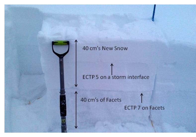
Over the past three days a heav load was deposited on a very weak foundation. Stability tests produced unstable results both within the storm snow and on the new snow/old snow interface. Dangerous avalanche conditions exist on Mt Ellis. Photo GNFAC
