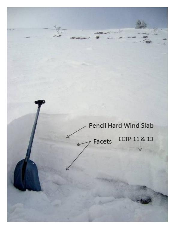
After 20" of fresh snow the snowpack on the Football Field was surprisingly thin. Not only was the pack thin, it was weak. During stability tests we got two ECT's to propagate on facets directly below a hard wind slab. This is discouraging since this area will continue to see loading and lots of traffic. Photo GNFAC
