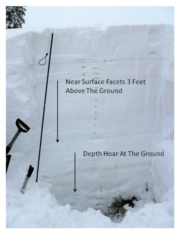
Two distinct weak layers exist in the snowpack near Lionhead. Both layers are fully capable of producing avalanches. Photo GNFAC
