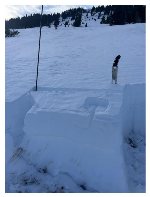
Dug a pit at 7600 ft on a NE facing slope. Full propagation on isolation of the column on the layer of concern about 16 inches down in this zone. Photo: Anonymous
