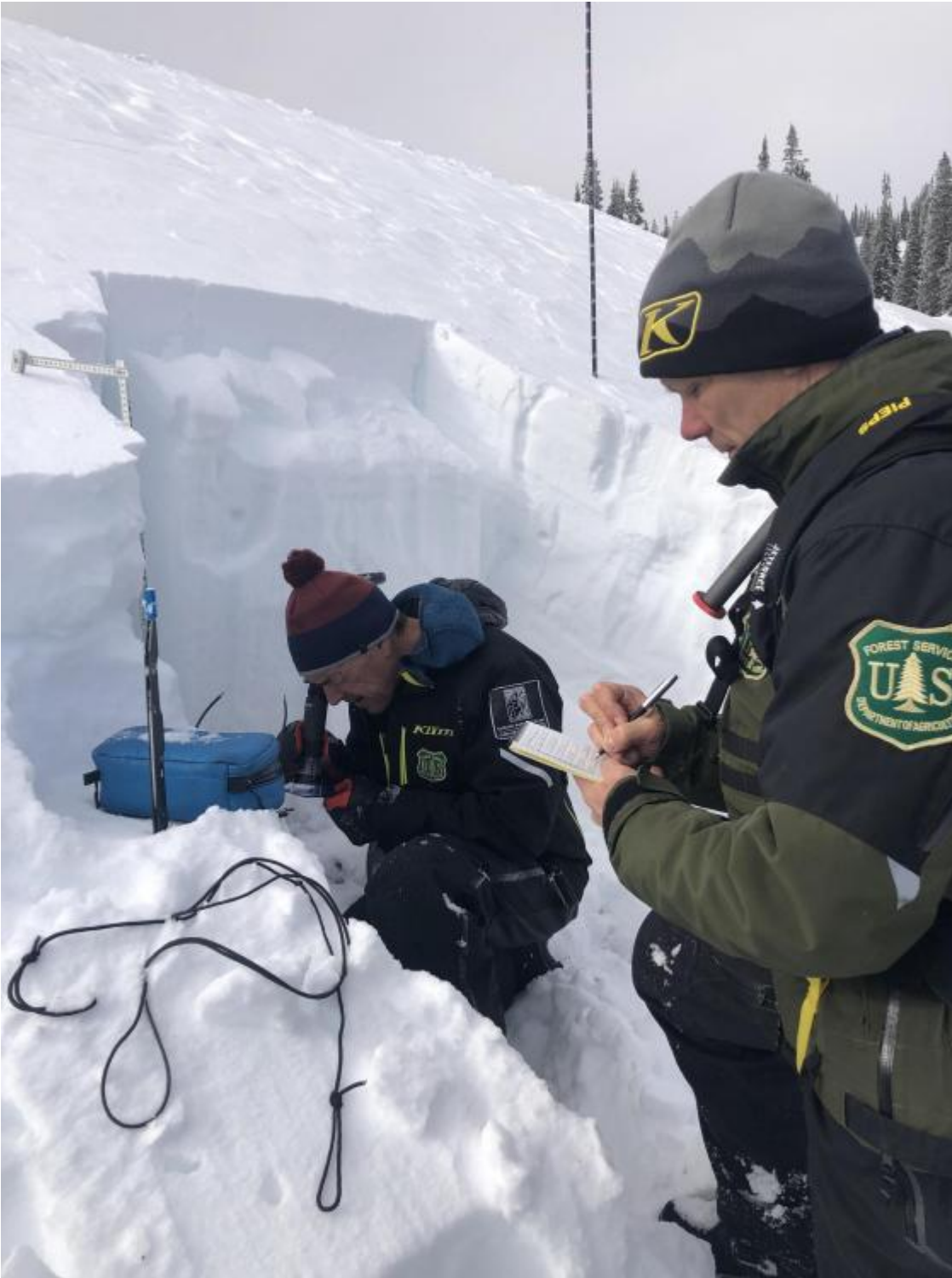
Identifying and recording grain types in the snowpack at the site of the Lionhead avalanche fatality. Photo: J. Norlander
