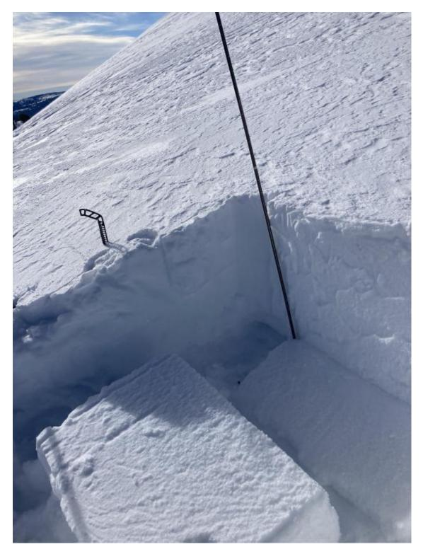
This test broke and propagated with some "extracurricular" hits in an extended column test in Beehive Basin. Photo: N Rustigian
