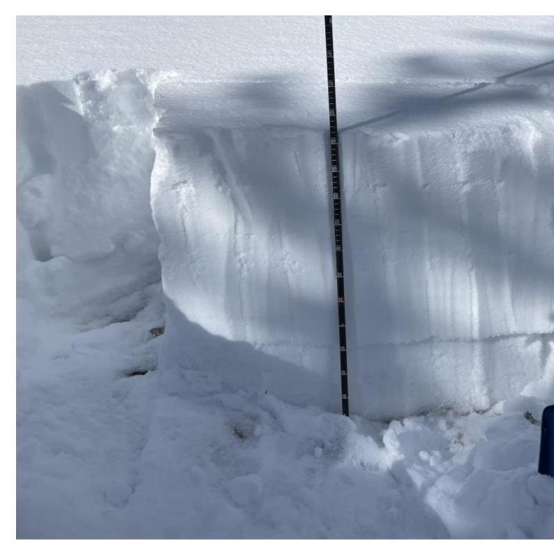
From e-mail 11/10/21: "an east aspect around 9900'. HS 63cms. ECTV on facets at 19cms." In this snowpit the slab collapsed above the weak layer when the observer isolated the column to perform an extended column test (ECT), hence the score ECTV (ECT-very easily collapsed and propagated). Photo: B. Fredlund
