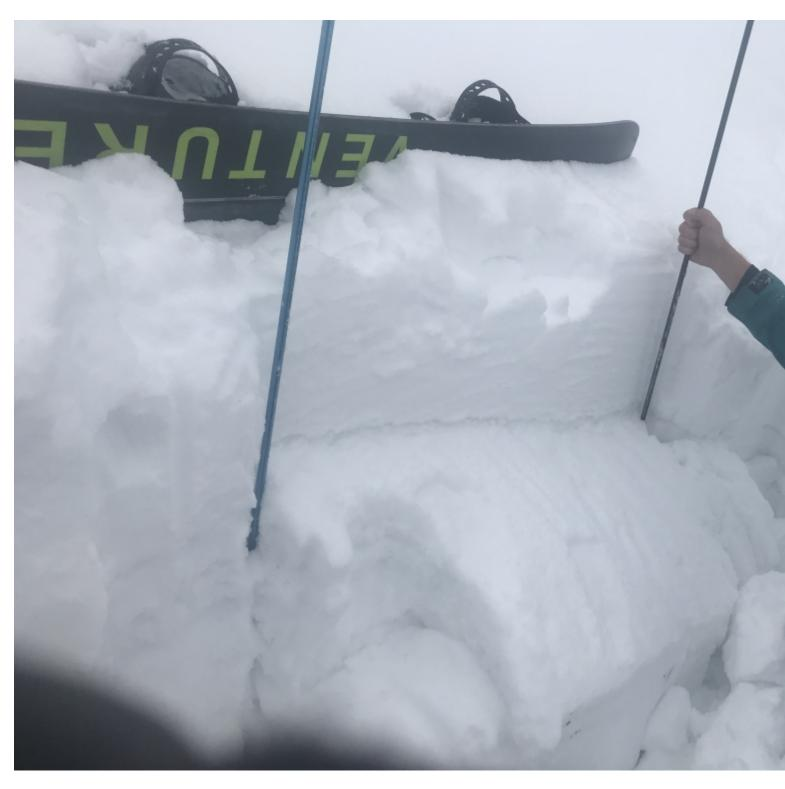
This snowpit was dug near the top of the Apron at Bridger Bowl. The stability test score of ECT 9 means it propogated all the way across and slid quickly on the 9th tap. The weak layer was 30 cm from the surface in a 90cm snowpack. The interface between the old/new snow may remain unstable through the weekend, especially with wind-loading. Photo: Roy Taylor
